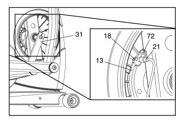
Then, retighten the M4 x 16mm Screw (72). Turn one of the Crank Arms (31) for a moment. Repeat until the console displays correct feedback. When the Reed Switch is correctly adjusted, replace the crank arm cover.
